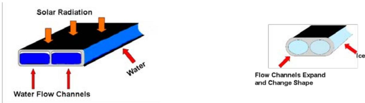
Although we advise draining a system before temperatures drop below freezing, we know that weather conditions can often change rapidly and this is not always possible. Because water expands by approximately 9 % when turning to ice, the strain put on a solar pool heating system can be devastating. Techno-Solis collectors are designed to withstand internal freezing because of their extra thick channel walls and elliptical shaped flow tubes that can expand and change shape.
