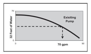
Choose the minimum and maximum flow rates based on Turnover Rate and Water Velocity and calculate the corresponding friction loss using the formula above. Plot each combination of friction loss and flow to create the system curve.
