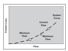
The point where the performance curve for a particular pump intersects the system curve determines the flow and Total Dynamic Head where that pump will operate.
